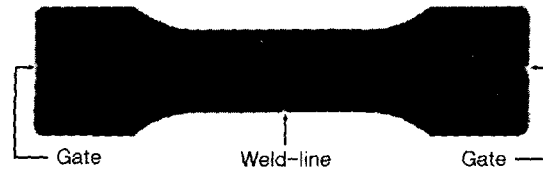
Fig. 1 Soft X-ray photography of products after injection molding
