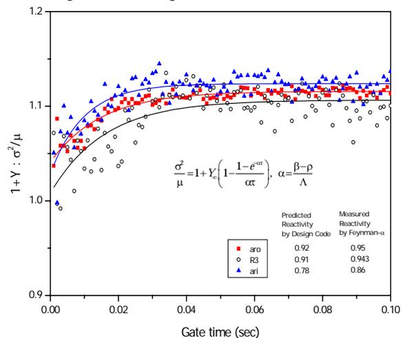
Fig. 5 VTMR variations and reactivities measured at the initial core of a KSNP
