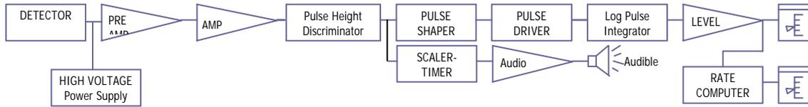
Fig. 2. The diagram for excor detector signal processing
