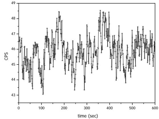
Fig 3. Measured pulse counts history in a WH reactor
