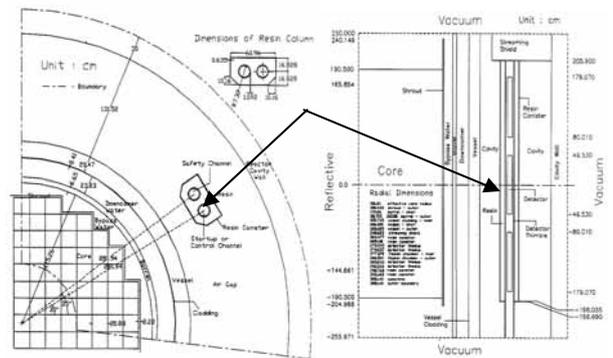
Fig. 1 Locations of source range detector in KSNP
