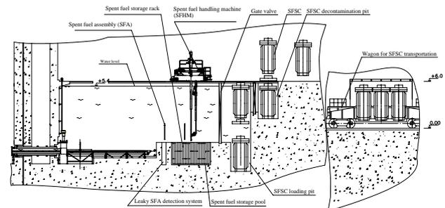
Figure 1. Spent fuel storage and handling scheme
