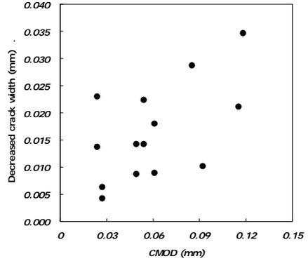
Figure 3 Decreased crack width due to self-healing
