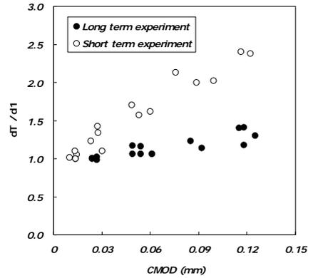
Figure 5 Relative penetration depth vs. CMOD
