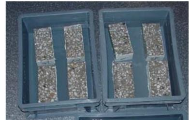
Figure 1 Immersion testing
