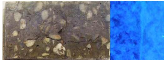
(b) Long term ex. (left: Cl<sup>-</sup> profile, right: crack picture)
