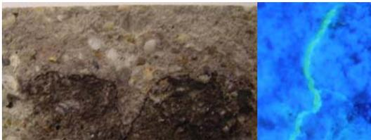
(a) short term exp.(left: Cl<sup>-</sup> profile, right: crack picture)
