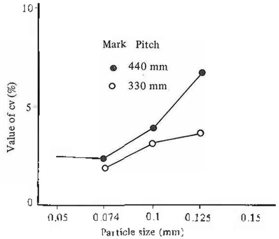
Figure 9. The effect of particle size on value of cv.
