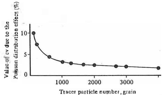
Figure 5. The effect of tracer particle number on coefficient of variation.
