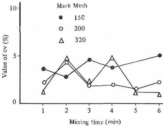
Figure 8. The curve of uniformity of 440 mm-pitch rotor.
