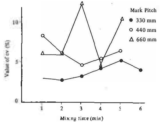
Figure 6. The effect of tracer particle number on uniformity of mixing.
