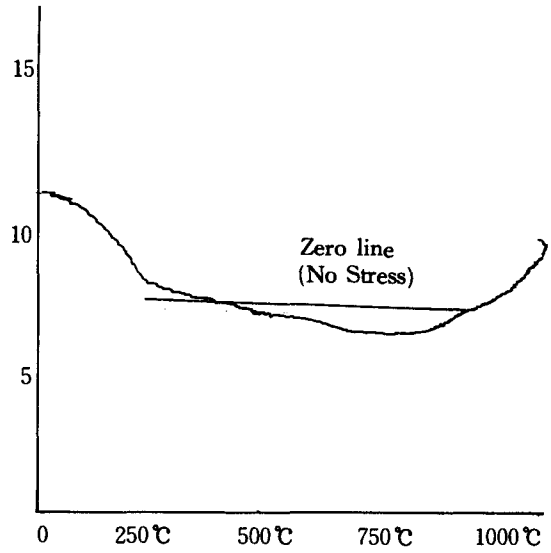
Fig. 9 Measurement of Stresses in glaze No. 13
