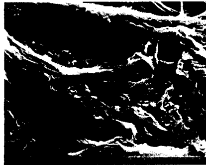
Photo. 2 Scanning electron micrographs of refined cotton linter fiber treated with waste cellulase
