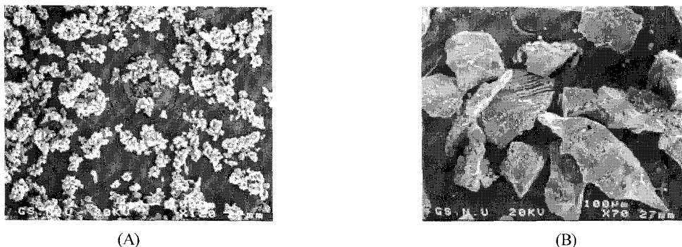
Figure 2. The SEM photograph of EPDM scrap: (A) grinding method, (B) cutting method.
