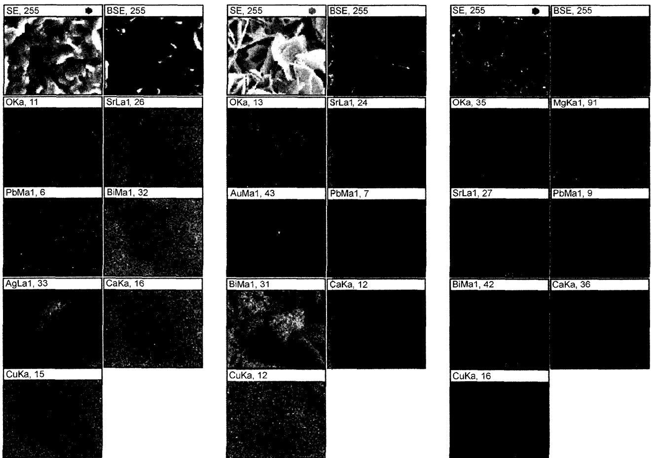
(a) Bi_{1.84}Pb_{0.34}Sr_{1.91}Ca_{2.03}Cu_{3.06}O_{10+δ} + Ag 50 wt% (b) Bi_{1.84}Pb_{0.34}Sr_{1.91}Ca_{2.03}Cu_{3.06}O_{10+δ} + Au 50 wt% (c) Bi_{1.84}Pb_{0.34}Sr_{1.91}Ca_{2.03}Cu_{3.06}O_{10+δ} + Mg 50 wt% Fig. 4. Secondary electron image and X-ray intensity maps of the surface of (a) Bi-2223+AgO 50 wt%, (b) Bi-2223+ Au_2O_3 50 wt%, and (c) Bi-2223+MgO 50 wt%.
