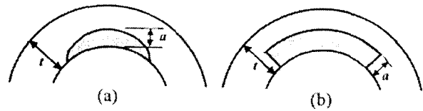
Fig. 2 Crack dimension and shape (a) a semi-elliptical crack, (b) a rectangular (constant depth) crack
