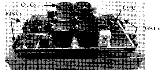
Fig. 9 Assembled component appearance in the transformer primary side high frequency inverter of soft switching PWM dc-dc converter circuit
