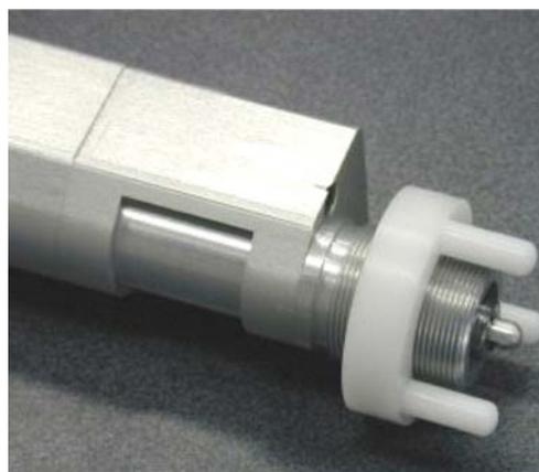
Fig. 2. The tactile sensor tip (arrow) which is placed and moved on the material to be measured.
