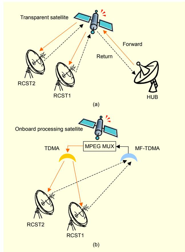
Fig. 2. Bent pipe satellite system vs. satellite system with OBP.
