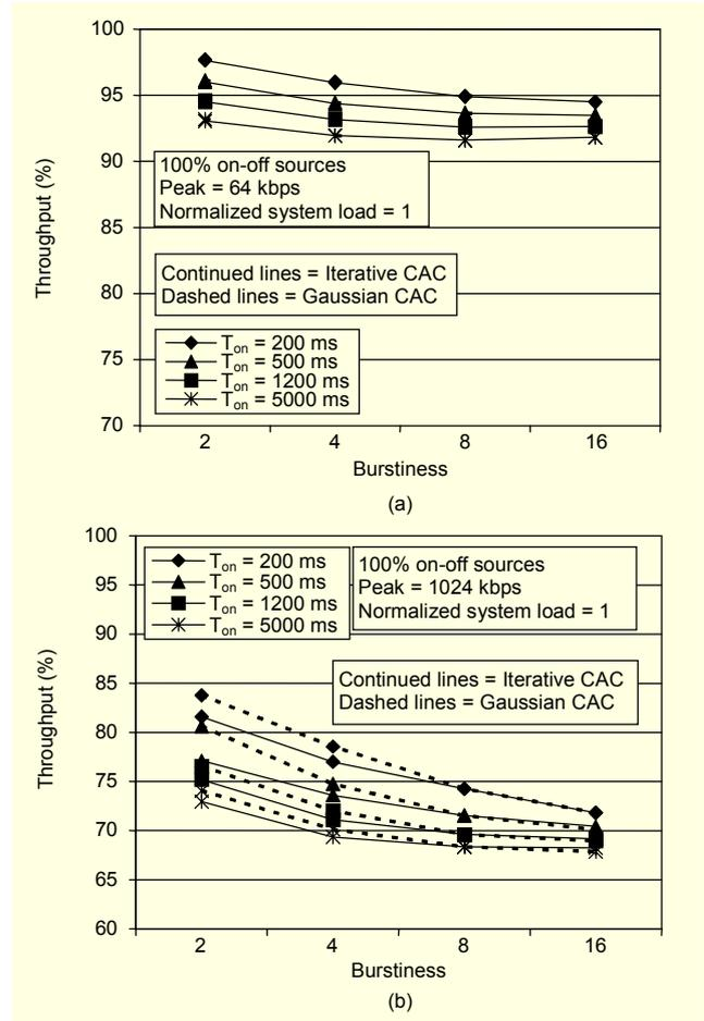
Fig. 12. System throughput over the return link: (a) PDR = 64 kbps and (b) PDR=1024 kbps.
