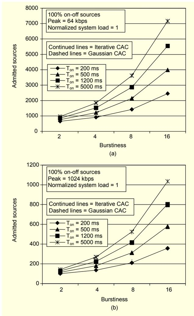
Fig. 11. Admitted sources over the return link: (a) PDR = 64 kbps and (b) PDR=1024 kbps.
