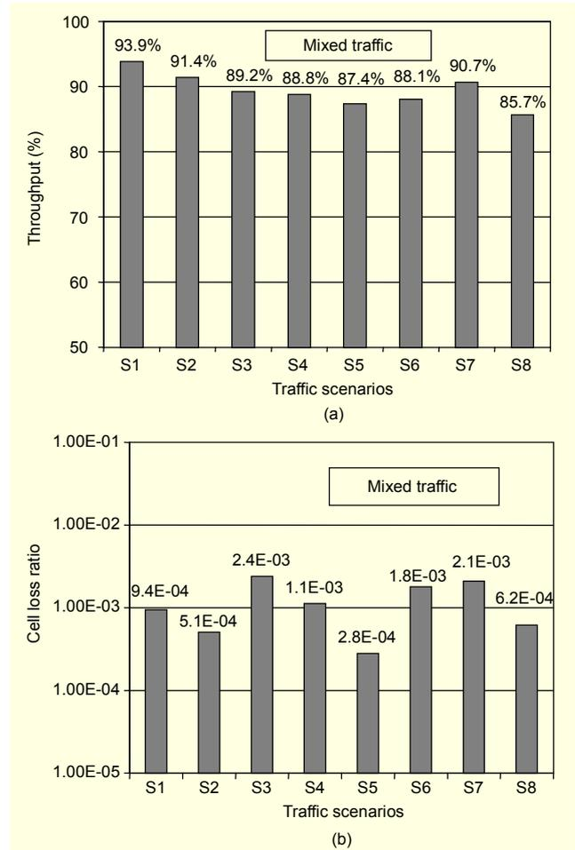
Fig. 8. (a) Return link throughput and (b) cell loss ratio in mixed condition.
