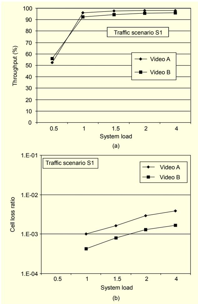
Fig. 7. (a) Return link throughput and (b) cell loss ratio for video traffic sources.
