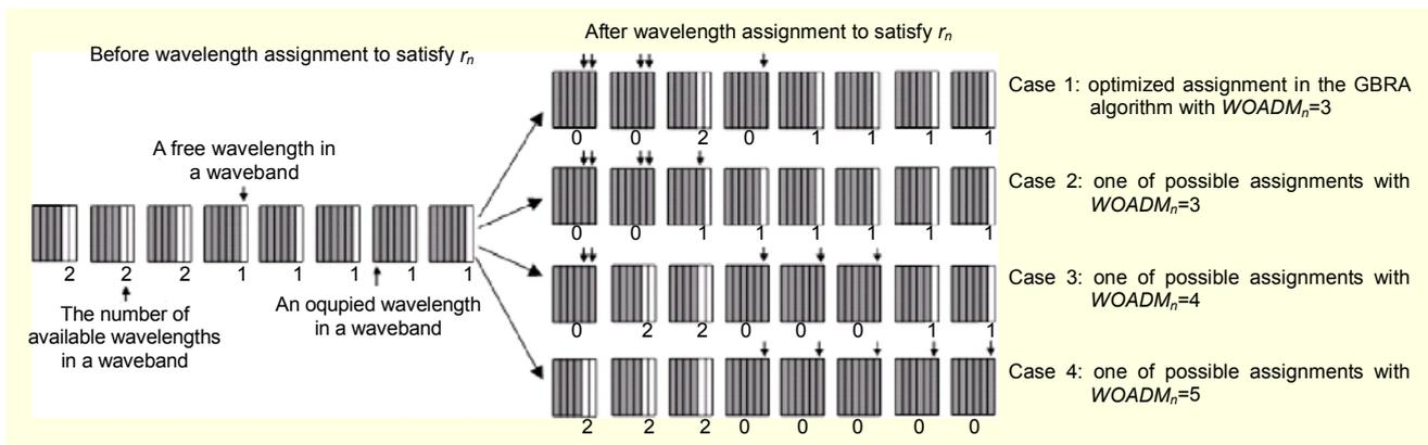
Fig. 4. The process of selecting available wavelengths of nonempty wavebands to satisfy  $r_n$ .
