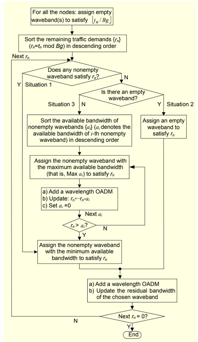
Fig. 3. Flowchart for the GBRA algorithm.
