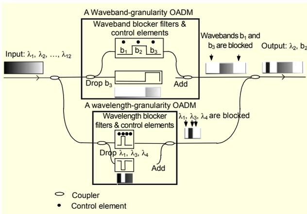
Fig. 2. The architecture of two-level parallel multi-granularity OADM node and a sample of  $\lambda_1, \lambda_3,$  and  $\lambda_4$  in  $b_1$  and  $b_3$  to be dropped in the OADM node.
