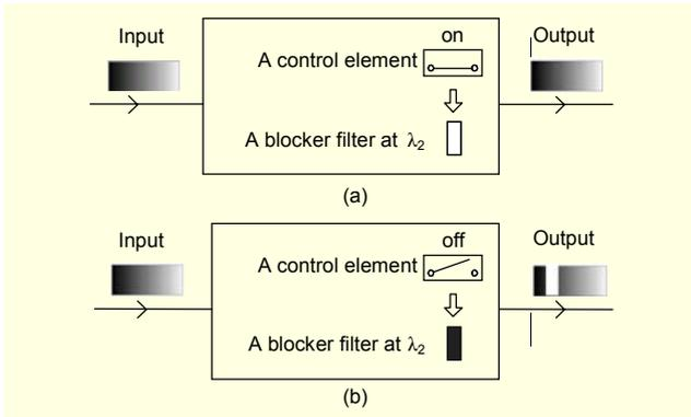
Fig. 1. Illustration of a blocker-filter controlled by a control element (a) a control element is in the on state and (b) a control element is in the off state.
