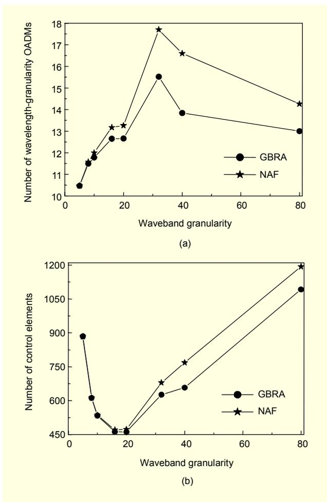
Fig. 5. 13-node ring network with 320 wavelengths (a) the number of wavelength-granularity OADMs, and (b) the number of control elements.
