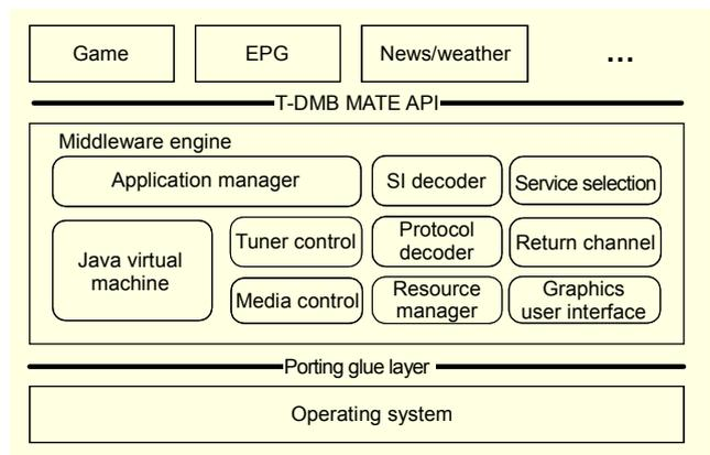
Fig. 3. The structure of the T-DMB MATE.
