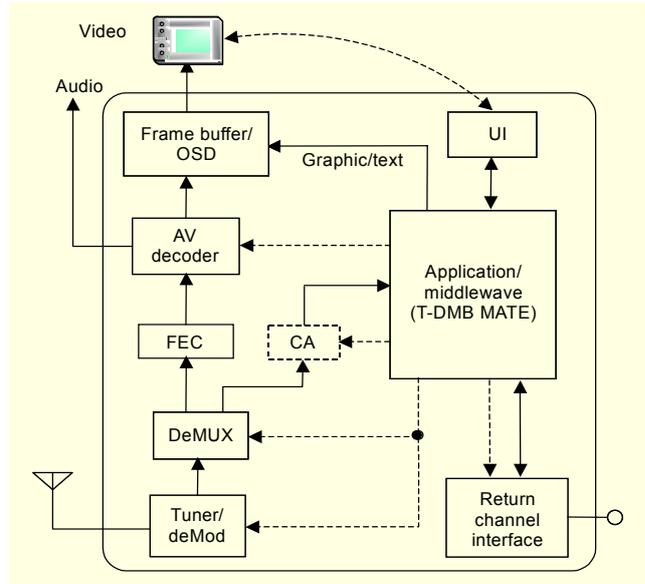
Fig. 2. The T-DMB receiver for the T-DMB MATE applications.
