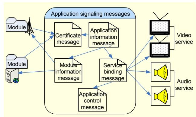
Fig. 5. Application signaling messages for application provision.
