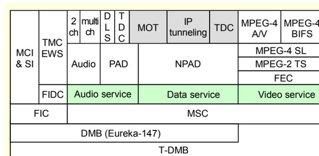
Fig. 1. The broadcasting protocol stack of T-DMB.
