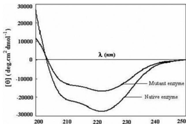
**Fig. 2.** Far-UV CD spectra of native and mutant bacterial luciferase in 50 mM-phosphate and 10 mM 2-mercaptethanol (pH 7) at 25°C.
