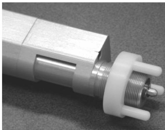
Fig. 2. The tactile sensor tip (arrow) which is placed and moved on the tissue surface to be measured
