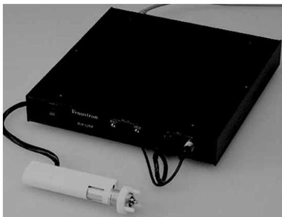
Fig. 1. The tactile sensor system (Venustron<sup>®</sup>, Axiom Co. Ltd., Japan) used for this study.
