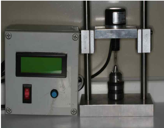
Fig. 1. Custom-made digital measuring device used to access rotational freedom.
