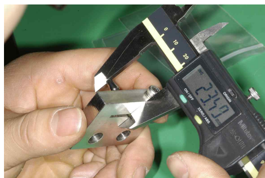
Fig. 8. Measurement of implant length.
