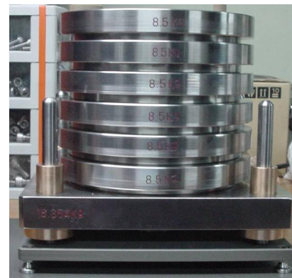
Figure 2. A schematic diagram and a picture of a compression set tester under constant load: ① weight and ② sample.
