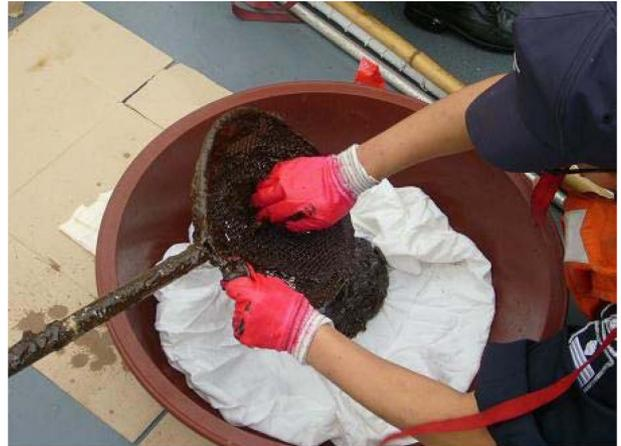
Fig. 3. A mesh scoop and the collected tar balls on the sea.
