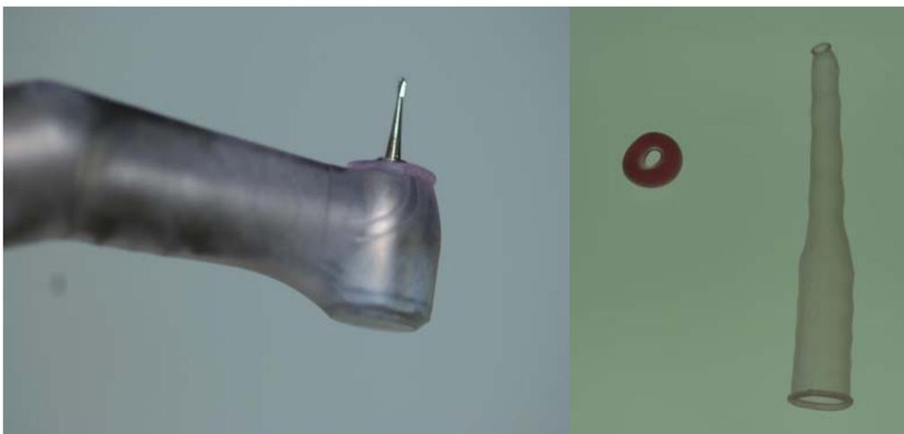
Fig. 1. Latex cover (Orokeeper<sup>®</sup> Orobiotech Co.,Korea) used in this study. Handpiece equipped with latex cover(left) and latex cover unrolled completely(right).
