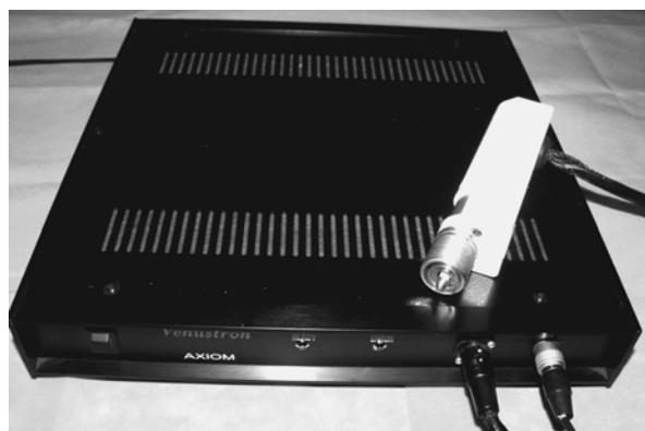
Fig. 1. The tactile sensor system(Venustron<sup>®</sup>, Axiom Co Ltd, Japan).
