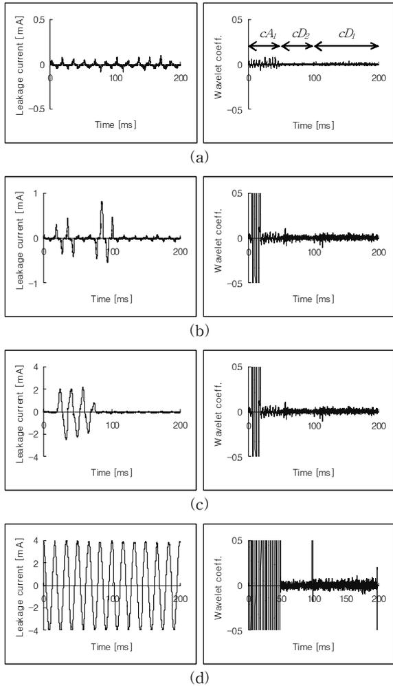
**Fig. 2** Transition of leakage current waveforms and their wavelet transforms. (a) Initial stage, (b) Middle stage, (c) Just prior to flashover stage, and (d) Flashover stage.
