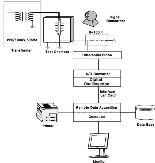
Fig. 1 The whole system diagram
