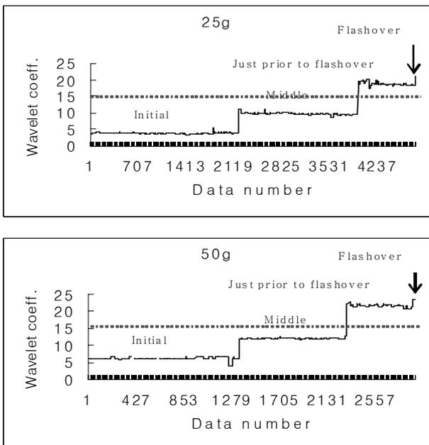
Fig. 4 Final results when using detail  $cD_1$  under 25g and 50g salt fogs
