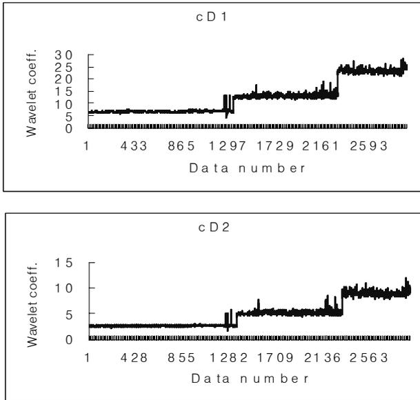
Fig. 3 Summation of details  $cD_1$  and  $cD_2$  under 50g salt fog.
