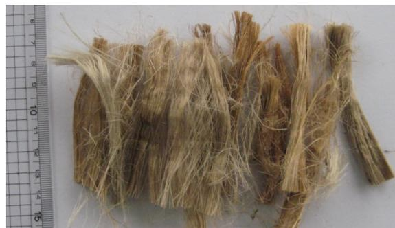
**Figure 1.** Photograph of chopped natural kenaf used in this study.
