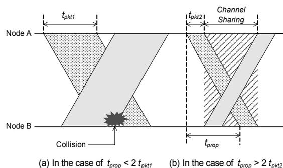
Fig. 1. Bi-directional transmission between two nodes.
