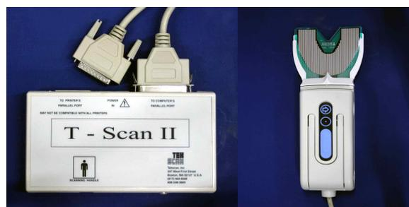
**Fig. 1.** T-Scan II (Tekscan, Boston, MA, U.S.A) parallel interface module and handle assembly
