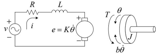
Fig. 2. Diagram of DC motor
