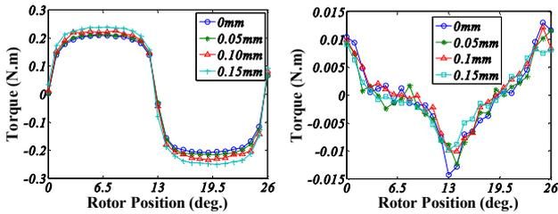
(a) Torque of  $P_A$  at  $i_A=2A$  (b) Torque of  $P_{xp}$  at  $i_{xp}=2A$
