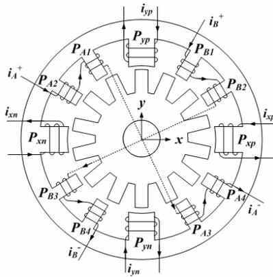
Fig. 4. Structure of proposed BLSRM
