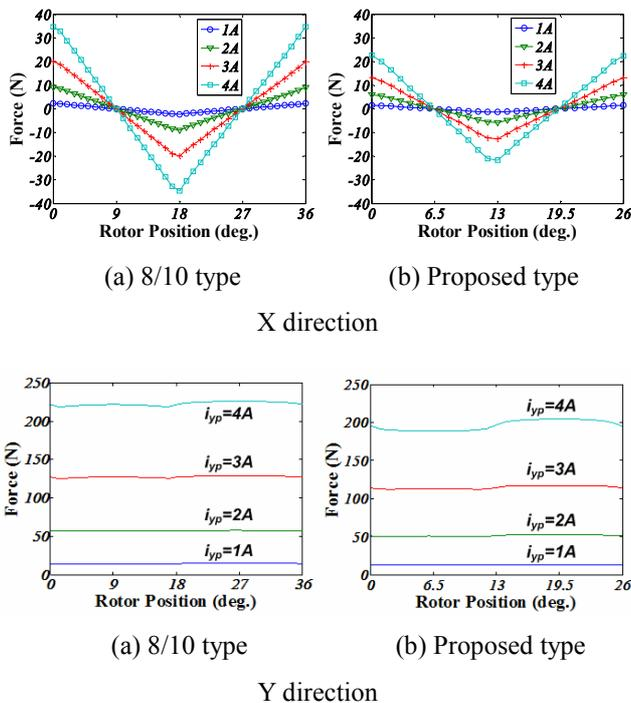
Fig. 12. Suspending force profiles of suspending force windings
