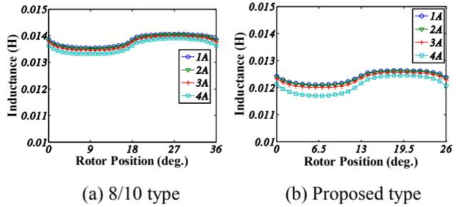
**Fig. 9.** Inductance profiles of suspending force windings
