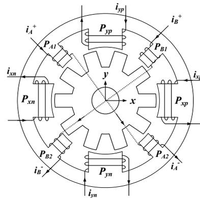
Fig. 3. Structure of 8/10 hybrid stator pole BLSRM
