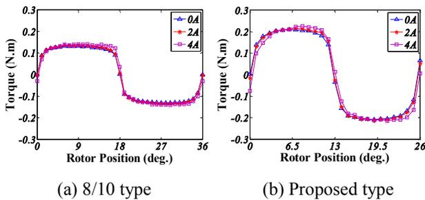
Fig. 11. Torque profiles with fixed torque current ( $i_A=2A$ ) and various suspending force currents
