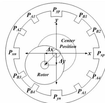
Fig. 14. Eccentricity effect of the air-gap displacement
