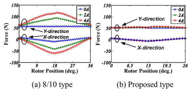
Fig. 13. Suspending force profiles with fixed suspending force current 2A and various torque currents
