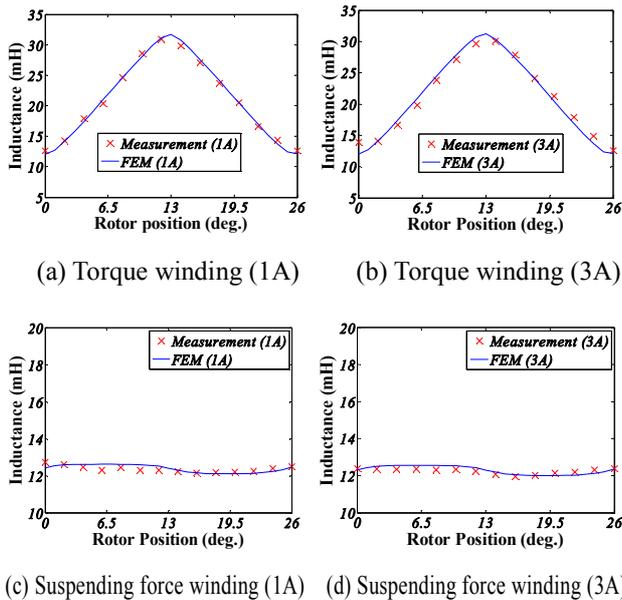
Fig. 19. Inductance: measured and FEM analytical result
