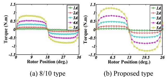
**Fig. 10.** Torque profiles of torque windings
