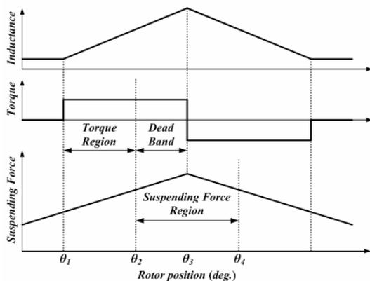
Fig. 2. Inductance, torque and suspending force profiles of general SRM
