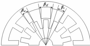
Fig. 5. Pole arc angles of the proposed BLSRM
