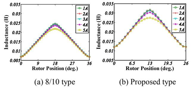
**Fig. 8.** Inductance profiles of torque windings
