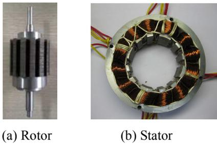
Fig. 18. Prototype of proposed BLSRM
