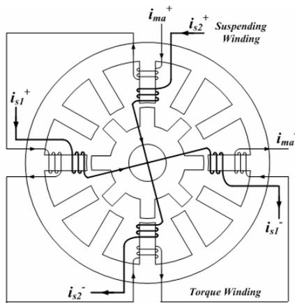
Fig. 1. Typical conventional BLSRM structure
