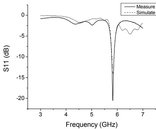
Fig. 5. Return loss of the antenna on the body
