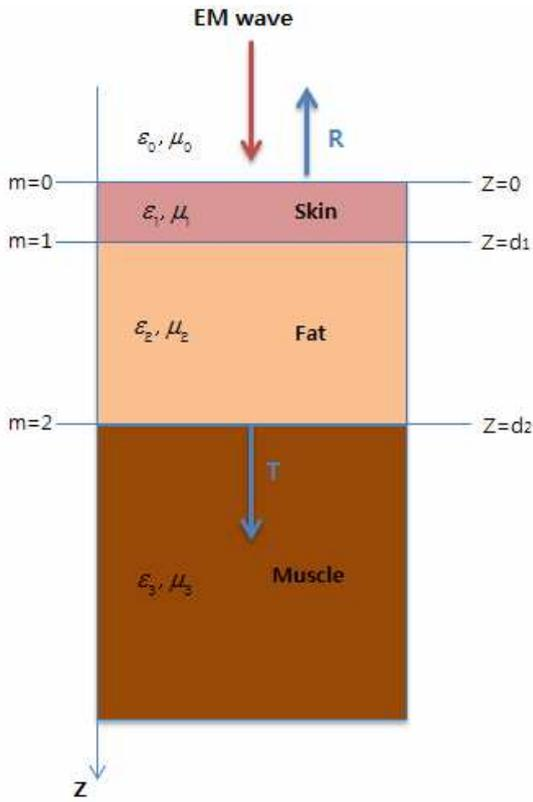
Fig. 1. Body Model with the Incident Wave
