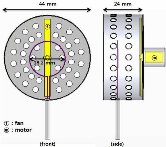
Fig. 4. Waveguide antenna with cooling system: (a) Front; (b) Side
