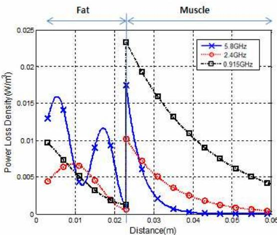
Fig. 2. Power Loss Density of Body Model
