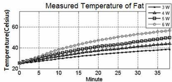
Fig. 7. Temperature curve of the fat with different input power
