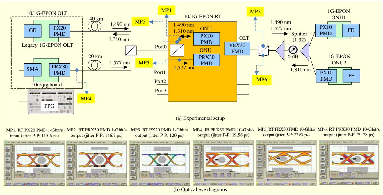
Fig. 8. Experimental setup and results at 10/1G-EPON RT.
