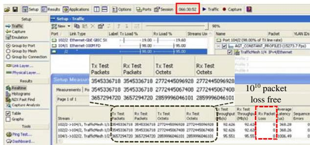
Fig. 10. Result of a long-term PER test.
