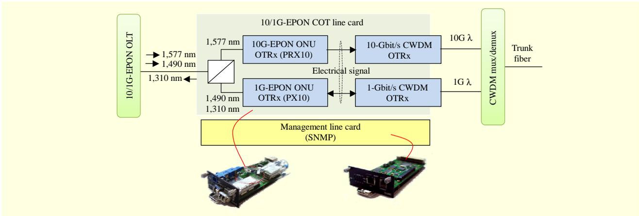
Fig. 3. Internal architecture of 10/1G-EPON COT line cards.
