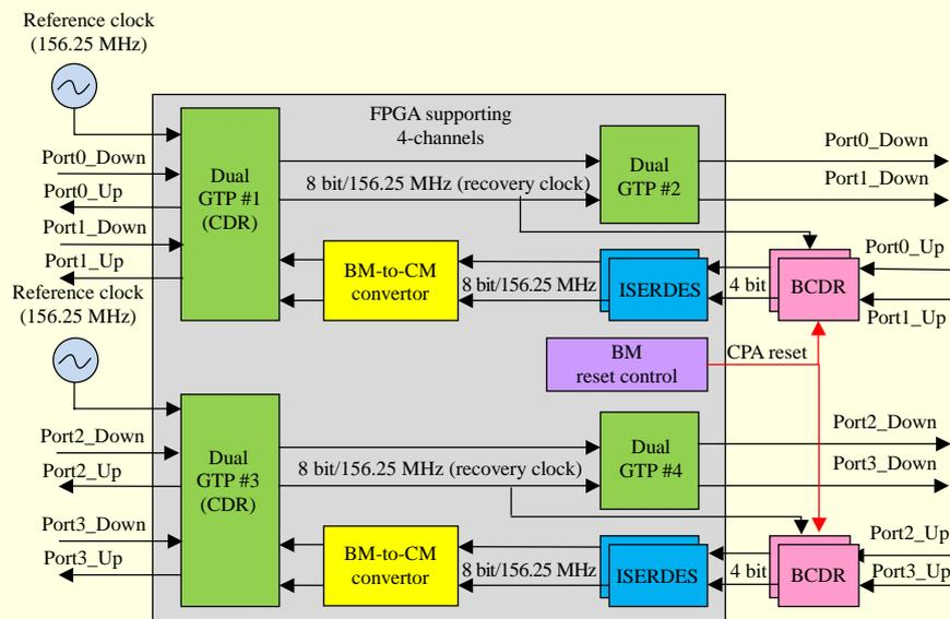
Fig. 5. Internal structure of FPGA for 3R-based signal regeneration [10].
