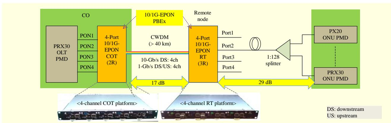
Fig. 2. 10/1G-EPON link structure using proposed hybrid-type PBEx.
