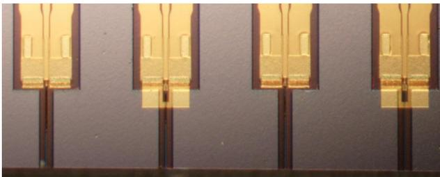
Fig. 5. Photography of fabricated TWPDs.
