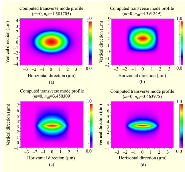
Fig. 2. Eigen-mode 2D profiles of waveguides for (a) lensed fiber with 3- $\mu\text{m}$  beam diameter, (b) 0.1- $\mu\text{m}$  core layer with subsidiary layers, and (c) 0.1- $\mu\text{m}$  and (d) 0.2- $\mu\text{m}$  core layers only.
