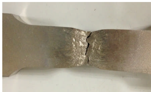
Fig. 4 Tensile test results of Ti
