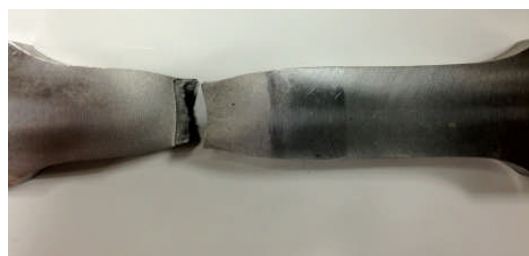
Fig. 5 Tensile test results of SM490A
