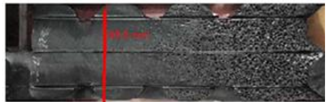
Figure 2. (a) Schematic diagram of the BPA measuring mold and (b) the blow point measured after 10 minutes-crosslinking.
