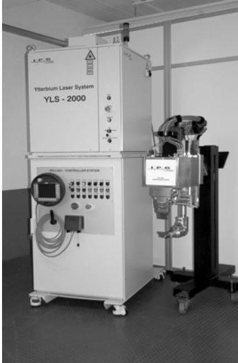
Fig. 10 LSS system consist of welding tool and integrated laser-controller cabinet. (footprint less than 1sqm)
