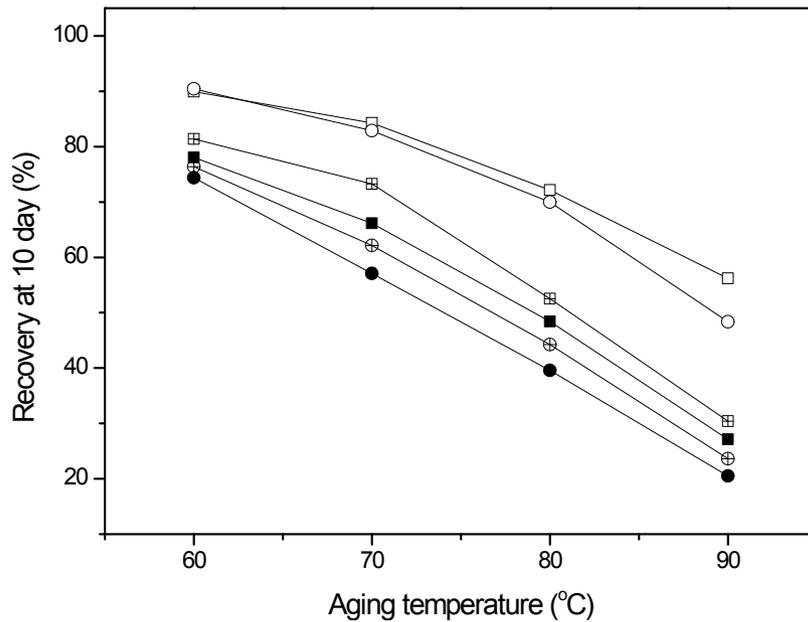
**Figure 6.** Variations of the limited recoveries (recoveries at the measurement time of 10 days) with the aging temperature. The squares and circles indicate the aging medium systems of the air to water (A→W) altering system and the water to air (W→A) altering system, respectively. The open, solid, and crossed symbols denote the filler systems of unfilled, carbon-filled, and silica-filled systems, respectively.
