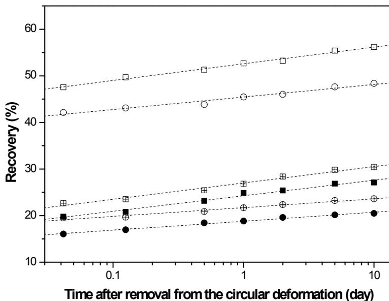
**Figure 5.** Recovery variations from the circularly deformed sample after thermal aging at 90°C with the measurement time. The squares and circles indicate the aging medium systems of the air to water (A→W) altering system and the water to air (W→A) altering system, respectively. The open, solid, and crossed symbols denote the filler systems of unfilled, carbon-filled, and silica-filled systems, respectively.
