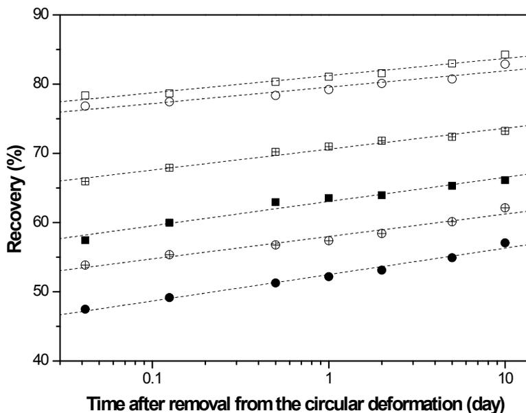
**Figure 3.** Recovery variations from the circularly deformed sample after thermal aging at 70°C with the measurement time. The squares and circles indicate the aging medium systems of the air to water (A→W) altering system and the water to air (W→A) altering system, respectively. The open, solid, and crossed symbols denote the filler systems of unfilled, carbon-filled, and silica-filled systems, respectively.
