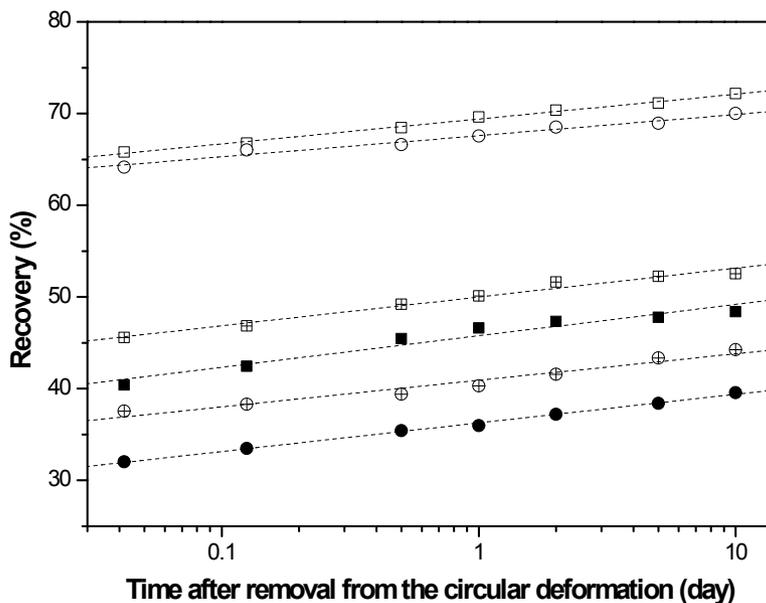
**Figure 4.** Recovery variations from the circularly deformed sample after thermal aging at 80°C with the measurement time. The squares and circles indicate the aging medium systems of the air to water (A→W) altering system and the water to air (W→A) altering system, respectively. The open, solid, and crossed symbols denote the filler systems of unfilled, carbon-filled, and silica-filled systems, respectively.
