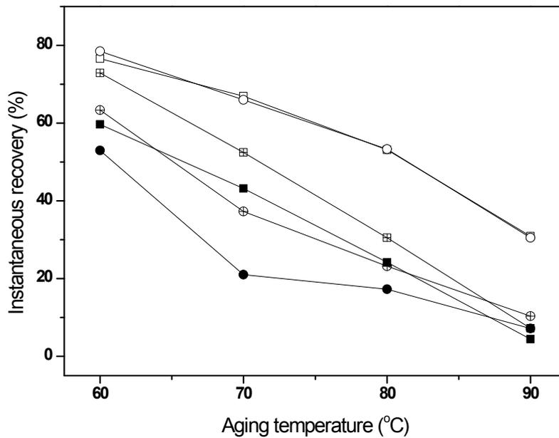
**Figure 7.** Variations of the instantaneous recoveries at  $10^{-6}$  day with the aging temperature. The squares and circles indicate the aging medium systems of the air to water (A→W) altering system and the water to air (W→A) altering system, respectively. The open, solid, and crossed symbols denote the filler systems of unfilled, carbon-filled, and silica-filled systems, respectively.
