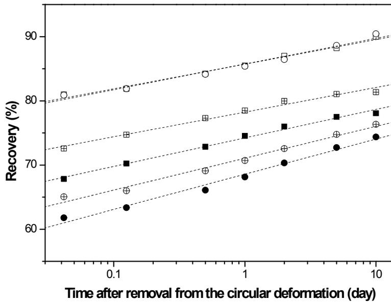
**Figure 2.** Recovery variations from the circularly deformed sample after thermal aging at 60°C with the measurement time. The squares and circles indicate the aging medium systems of the air to water (A→W) altering system and the water to air (W→A) altering system, respectively. The open, solid, and crossed symbols denote the filler systems of unfilled, carbon black-filled, and silica-filled systems, respectively.
