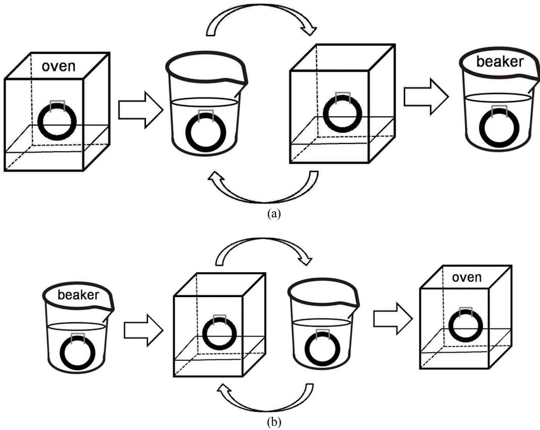
**Figure 1.** Altering aging medium systems of the circular deformation test. (a) the air to water altering system (A→W altering system, changing the medium each one day, the initial medium was air) and (b) the water to air altering system (W→A altering system, changing the medium each one day, the initial medium was distilled water).
