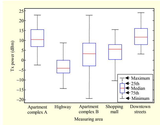
Fig. 5. Practical measurement of LTE UE transmitting power.
