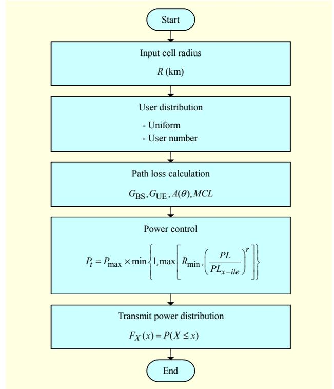
Fig. 3. Simulation flowchart for calculation of transmitting power.
