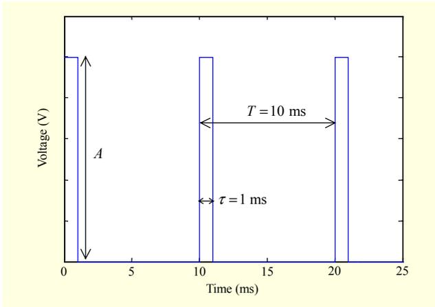
Fig. 1. LTE UE signal format in time domain.
