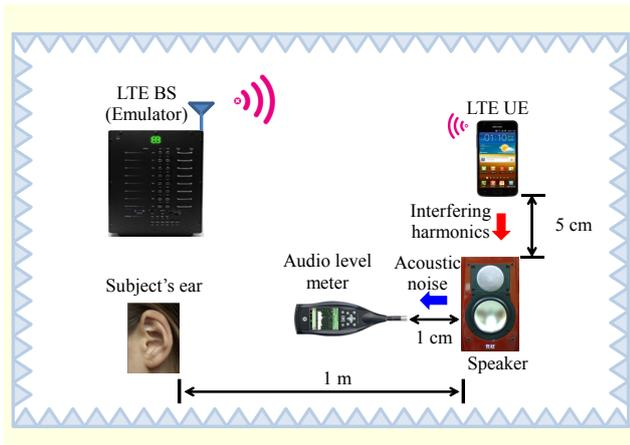
Fig. 6. Configuration of experiment.
