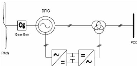
Fig. 3. Configuration of the DFIG
