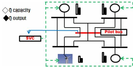
Fig. 7. Configuration of hybrid SVC
