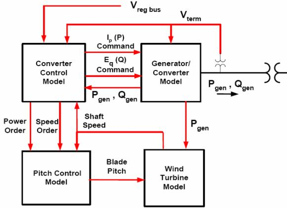
Fig. 5. Model block of the DFIG
