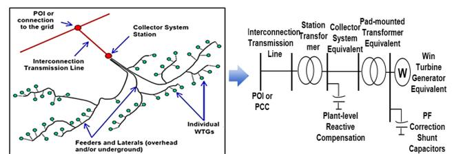
Fig. 4. Equivalent process of wind farms
