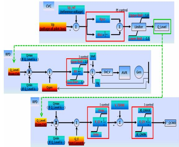
Fig. 6. Schematic of hybrid SVC
