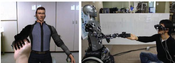
**Fig. 17.** An example of a tangible interaction between the human user and the TAV (*handshaking*)
