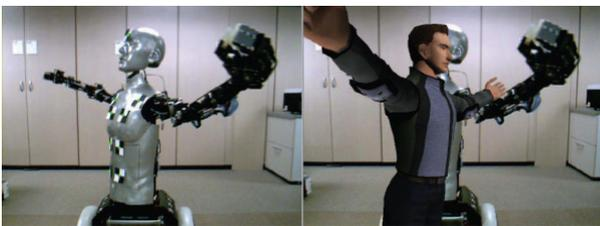
Fig. 12. Failure of tracking markers due to rapid motion of the TA
