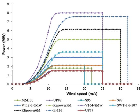
**Fig. 2.** Power curves of the 11 commercial WGs [13-21]
