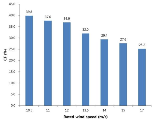
**Fig. 3.** Average CFs of the commercial WGs with the rated wind speed
