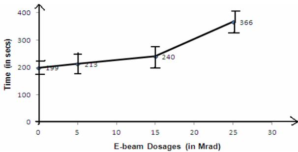
Fig. 7. Arc resistance of SiR-EPDM Blend
