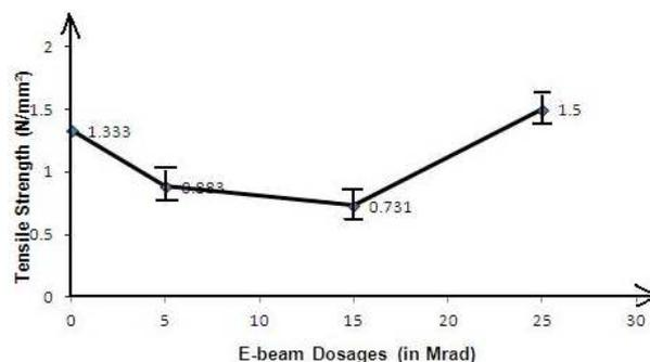
Fig. 4. Tensile strength of SiR-EPDM Blend
