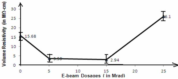
Fig. 6. Volume Resistivity of SiR-EPDM Blend
