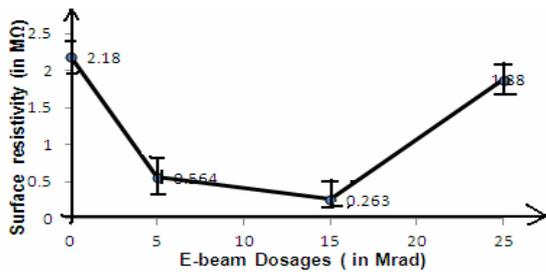
Fig. 5. Surface Resistivity of SiR-EPDM Blend
