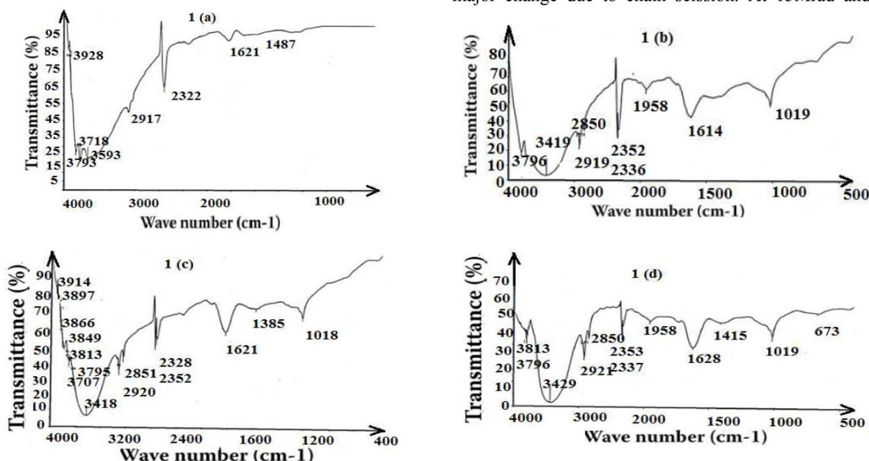
Fig. 1. FTIR Spectra SiR-EPDM Blend irradiated by various doses of E-beam: (a) 0 Mrad (virgin sample); (b) 5 Mrad; (c) 15 Mrad and (d) 25 Mrad
