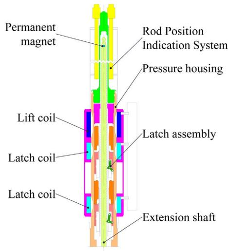
**Fig. 1.** (Color online) Schematic diagram of the CRDM.
