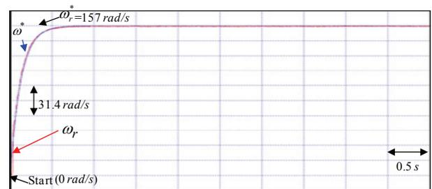
Fig. 19. Experimental result of speed tracking response using the hybrid recurrent Chebyshev NN control system for the V-belt CVT system driven by PMSM at 157 rad/s case
