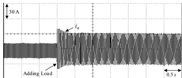
Fig. 32. Experimental result of measured current in phase  $a$  using the hybrid recurrent Chebyshev NN control system under  $T_l=2Nm(T_a)+T_{un}$  load torque disturbances with adding load at 314 rad/s case
