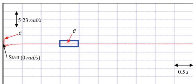
Fig. 20. Experimental result of speed tracking error using the hybrid recurrent Chebyshev NN control system for the V-belt CVT system driven by PMSM at 157 rad/s case
