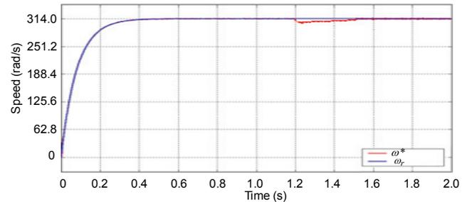
**Fig. 7.** Simulated result of speed tracking response using the hybrid recurrent Chebyshev NN control system for the V-belt CVT system driven by PMSM at 314 rad/s case with adding load torque disturbance  $T_l = 2Nm$  in  $t = 1.2$ sec
