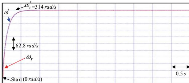
Fig. 23. Experimental result of speed tracking response using the hybrid recurrent Chebyshev NN control system for the V-belt CVT system driven by PMSM at 314 rad/s case
