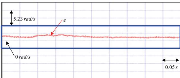
Fig. 17. Experimental result of speed tracking error amplification using the PI controller for the V-belt CVT system driven by PMSM at 314 rad/s case
