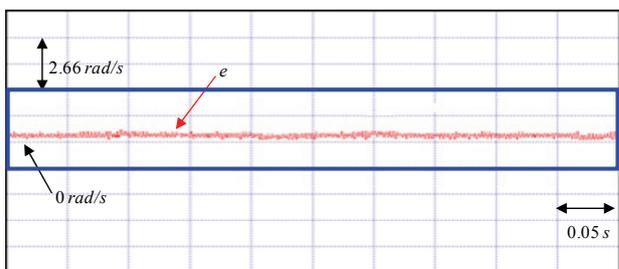
Fig. 21. Experimental result of speed tracking error amplification using the hybrid recurrent Chebyshev NN control system for the V-belt CVT system driven by PMSM at 157 rad/s case
