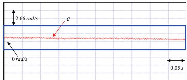
**Fig. 13.** Experimental result of speed tracking error amplification using the PI controller for the V-belt CVT system driven by PMSM at 157 rad/s case
