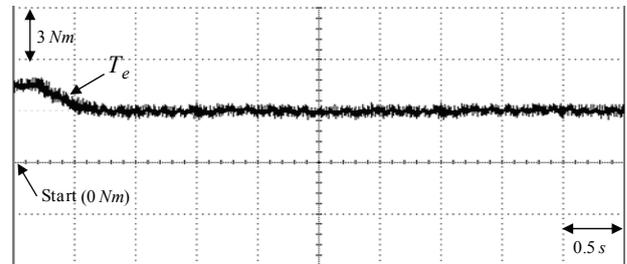
Fig. 26. Experimental result of command electromagnetic torque response using the hybrid recurrent Chebyshev NN control system for the V-belt CVT system driven by PMSM at 314 rad/s case
