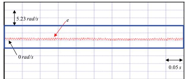
Fig. 25. Experimental result of speed tracking error amplification using the hybrid recurrent Chebyshev NN control system for the V-belt CVT system driven by PMSM at 314 rad/s case
