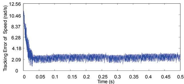
**Fig. 5.** Simulated results of speed tracking error using the PI controller for the V-belt CVT system driven by PMSM at 314 rad/s case with adding load torque disturbance  $T_l = 2Nm$  in  $t = 1.2$ sec
