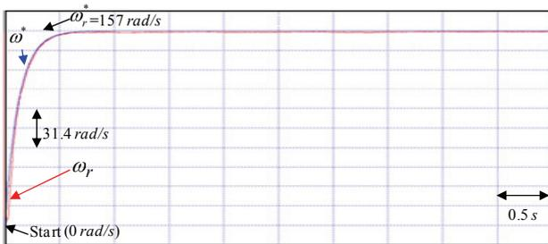
**Fig. 11.** Experimental result of speed tracking response using the PI controller for the V-belt CVT system driven by PMSM at 157 rad/s case
