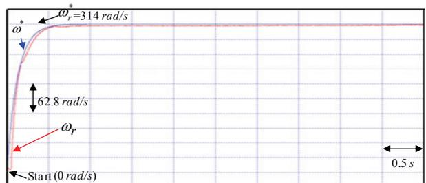
**Fig. 15.** Experimental result of speed tracking response using the PI controller for the V-belt CVT system driven by PMSM at 314 rad/s case
