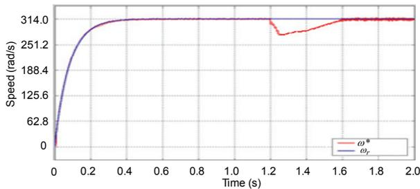
**Fig. 4.** Simulated result of speed tracking response using the PI controller for the V-belt CVT system driven by PMSM at 314 rad/s case with adding load torque disturbance  $T_l = 2Nm$  in  $t = 1.2$ sec
