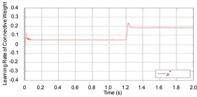
**Fig. 10.** Simulated results of learning rate  $\mu^*$  of connective weights in the recurrent Chebyshev NN at 314 rad/s with adding load torque disturbance  $T_l=2Nm$  in  $t=1.2sec$
