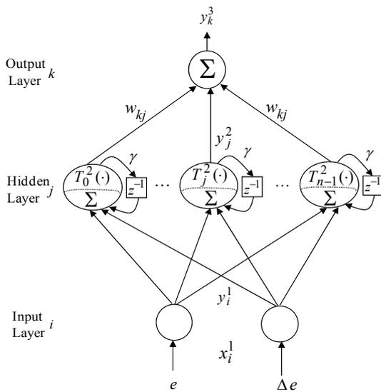
Fig. 3. Structure of the three-layer recurrent Chebyshev NN
