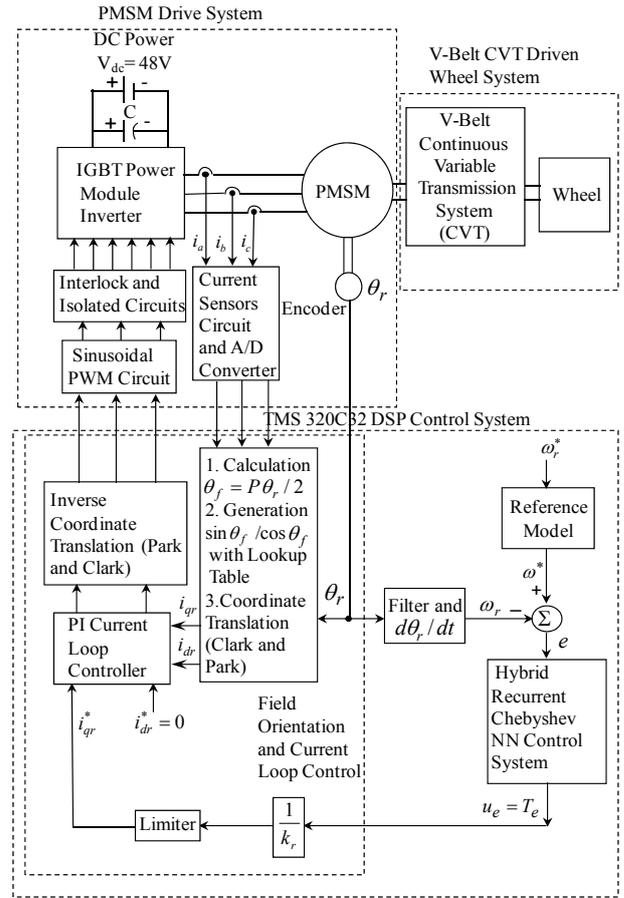
Fig. 1. Block diagram of the V-belt CVT system driven by PMSM
