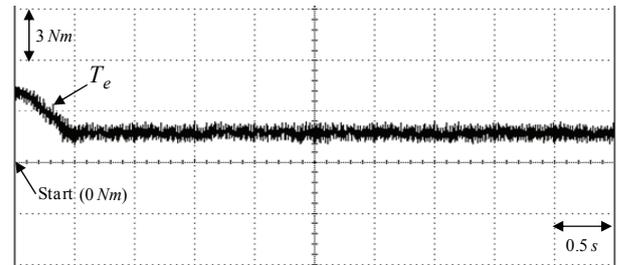
**Fig. 14.** Experimental result of command electromagnetic torque response using the PI controller for the V-belt CVT system driven by PMSM at 157 rad/s case
