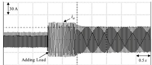
Fig. 30. Experimental result of measured current in phase  $a$  using the PI controller under  $T_l=2Nm(T_a)+T_{un}$  load torque disturbances with adding load at 314 rad/s case
