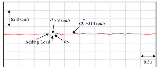
Fig. 31. Experimental result of speed response using the hybrid recurrent Chebyshev NN control system under  $T_l=2Nm(T_a)+T_{un}$  load torque disturbances with adding load at 314 rad/s case
