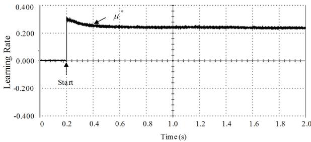
Fig. 28. Experimental result of optimal learning rate  $\mu^*$  of connective weights in the recurrent Chebyshev NN at 314 rad/s case
