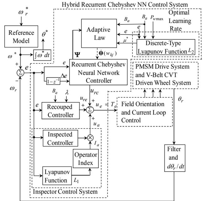
Fig. 2. Block diagram of the hybrid recurrent Chebyshev NN control system
