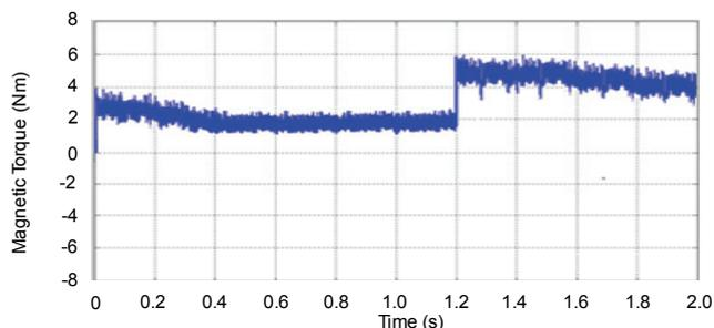
**Fig. 6.** Simulated result of command electromagnetic torque response using the PI controller for the V-belt CVT system driven by PMSM at 314 rad/s case with adding load torque disturbance  $T_l = 2Nm$  in  $t = 1.2$ sec
