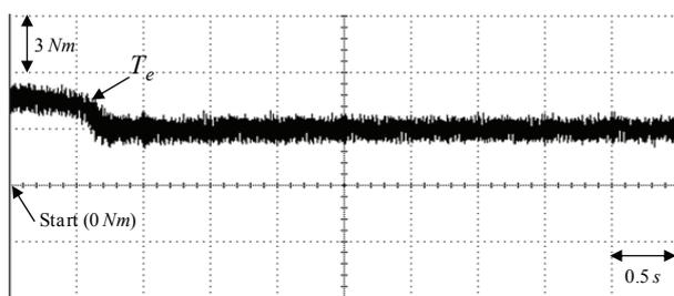
Fig. 18. Experimental result of command electromagnetic torque response using the PI controller for the V-belt CVT system driven by PMSM at 314 rad/s case
