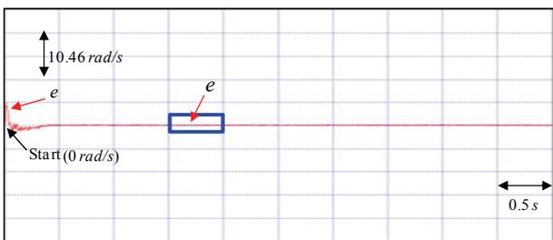
Fig. 24. Experimental result of speed tracking error using the hybrid recurrent Chebyshev NN control system for the V-belt CVT system driven by PMSM at 314 rad/s case
