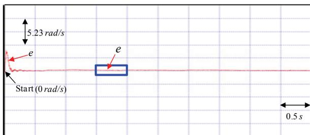
**Fig. 12.** Experimental result of speed tracking error using the PI controller for the V-belt CVT system driven by PMSM at 157 rad/s case
