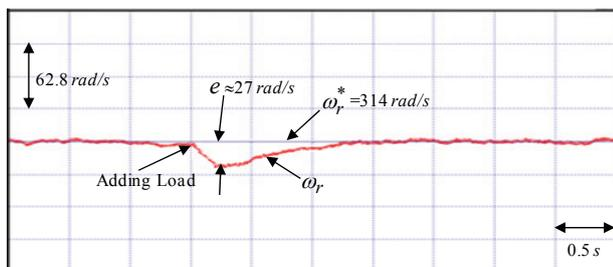
Fig. 29. Experimental result of speed response using the PI controller under  $T_l=2Nm(T_a)+T_{un}$  load torque disturbances with adding load at 314 rad/s case
