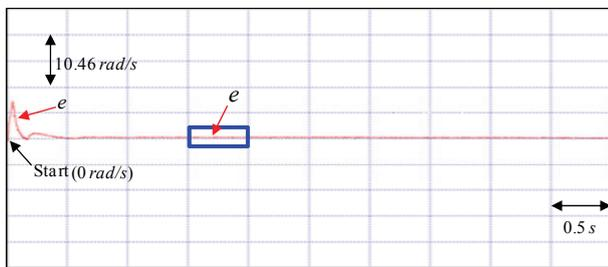
Fig. 16. Experimental result of speed tracking error using the PI controller for the V-belt CVT system driven by PMSM at 314 rad/s case
