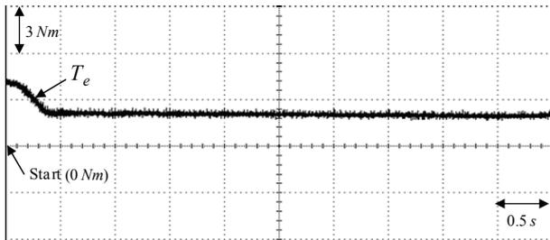
Fig. 22. Experimental result of command electromagnetic torque response using the hybrid recurrent Chebyshev NN control system for the V-belt CVT system driven by PMSM at 157 rad/s case
