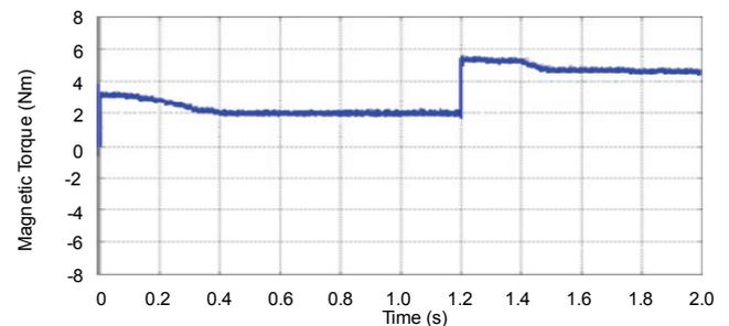
**Fig. 9.** Simulated result of command electromagnetic torque response using the hybrid recurrent Chebyshev NN control system for the V-belt CVT system driven by PMSM at 314 rad/s case with adding load torque disturbance  $T_l = 2Nm$  in  $t = 1.2$ sec
