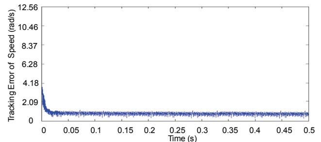
**Fig. 8.** Simulated results of speed tracking error using the hybrid recurrent Chebyshev NN control system for the V-belt CVT system driven by PMSM at 314 rad/s case with adding load torque disturbance  $T_l = 2Nm$  in  $t = 1.2$ sec
