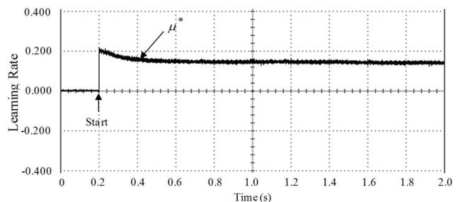
Fig. 27. Experimental result of optimal learning rate  $\mu^*$  of connective weights in the recurrent Chebyshev NN at 157 rad/s case
