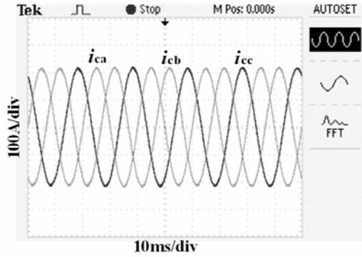
(a) the input currents of PWM rectifier
