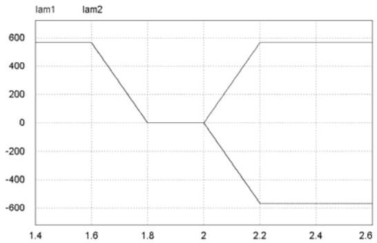
(a) the given amplitude of  $\alpha$ - and  $\beta$ -phase currents
