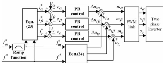
(a) the current composite control diagram of TPTLI
