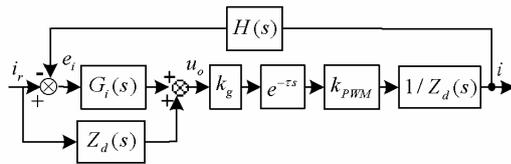
(b) the control block diagram of TPTLI in s domain
