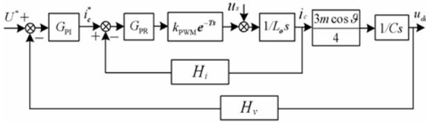
**Fig. 11.** The control block diagram for PWM link in  $s$ -domain
