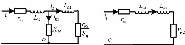
(a) the equivalent circuit (b) the simplified equivalent circuit
