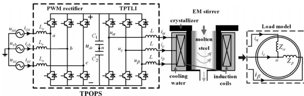
Fig. 1. The topology of TPOPS for EM stirring
