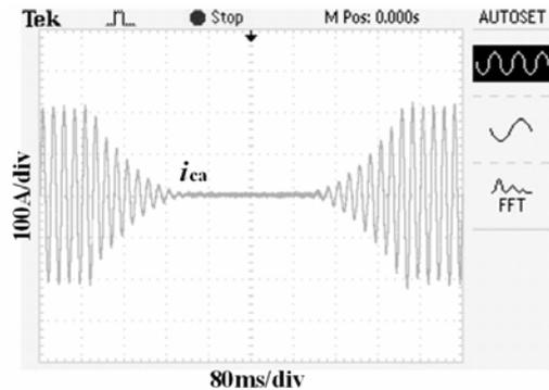
(b) the a-phase input current of PWM rectifier
