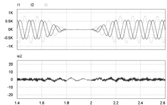
(c) the output currents with the proposed composite control method
