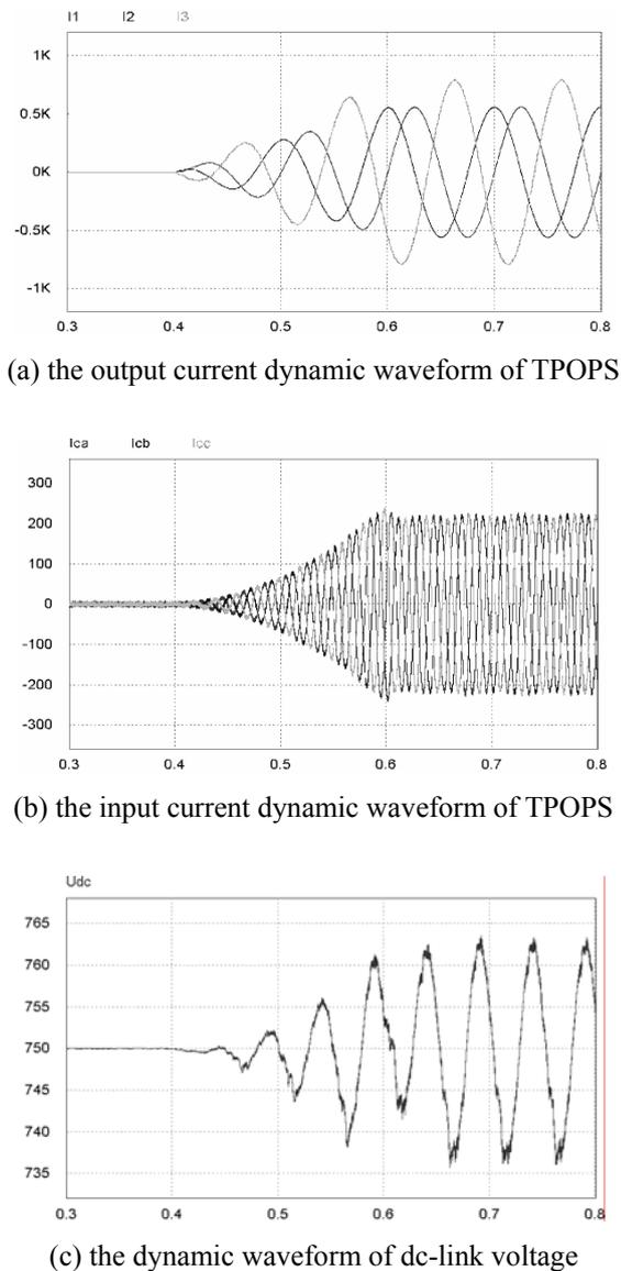
Fig. 5. The dynamical waveforms when switching into the EM stirring load
