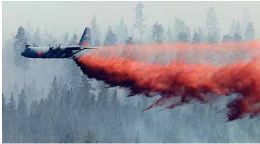
Fig. 3 MAFFS C-130 chemical fire retardant
