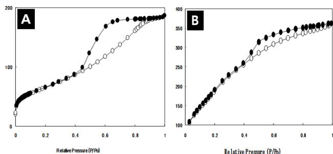
Figure 3. Nitrogen adsorption/desorption isotherms for starting hollow type mesoporous silica (A) and mesoporous hollow carbon capsules (B) templated by PS.
