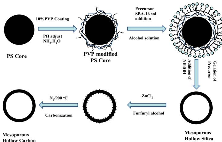
**Scheme 1. Fabrication of mesoporous carbons using PS template and SBA-16 silica-sol by sacrificial core method.**
