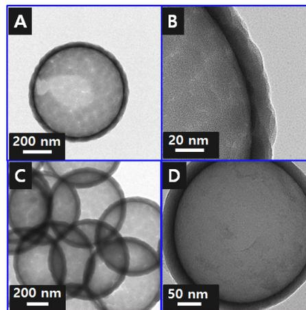
Figure 5. TEM images of hollow silica sphere (A, B) and hollow carbon spheres (C, D).
