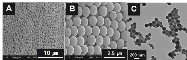
**Figure 1.** SEM (A, B) and TEM (C) images for PS micro beads used as a hard template for the fabrication of hollow mesoporous silica and carbon microcapsules.
