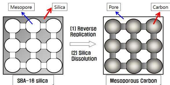
**Scheme 2.** Concept of mesoporous carbon formation from SBA-16 silica by reverse replication.
