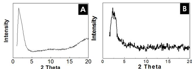
**Figure 2.** XRD pattern of hollow mesoporous silica sphere (A) and carbon microcapsule (B).
