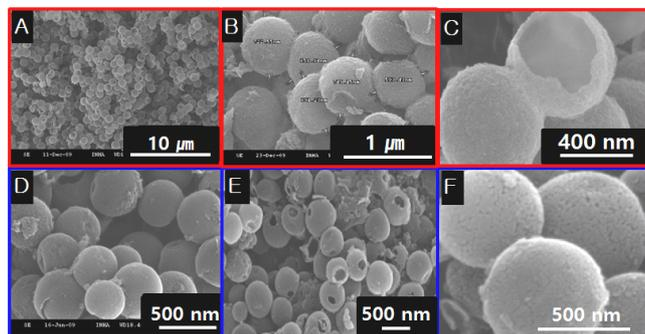
Figure 4. SEM images of mesoporous hollow silica spheres (A, B, C) and hollow carbon spheres (D, E, F).
