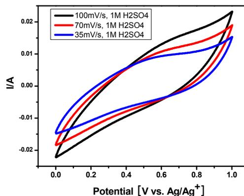
Figure 6. Cyclic voltammograms of hollow carbon spheres.
