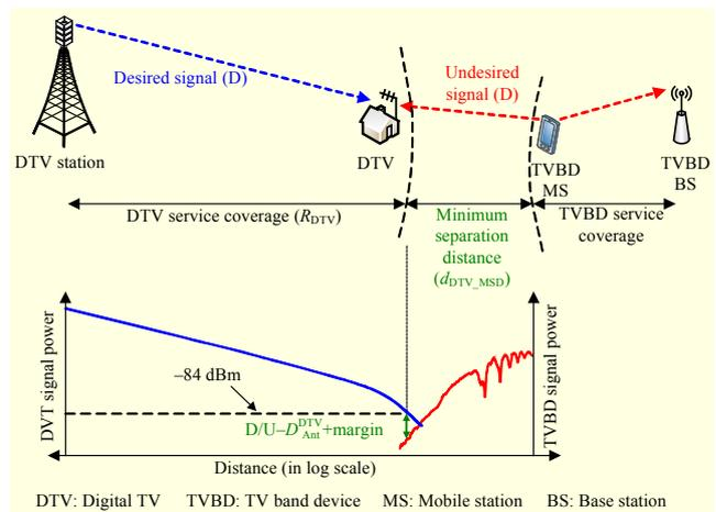
Fig. 1. Minimum separation distance of TVBD MS from edge of DTV service coverage (grade B contour).
