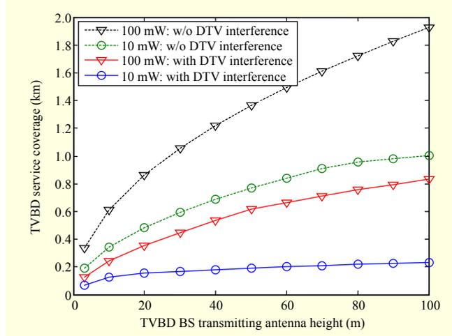
Fig. 9. Comparison of coverage reduction of TVBD network due to DTV interference with two different TVBD transmit power levels.
