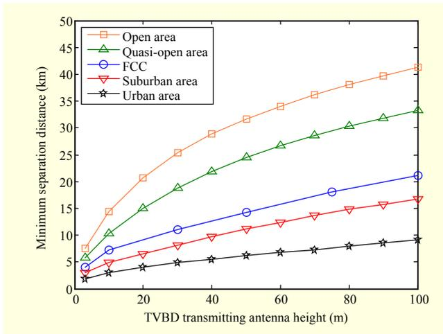
Fig. 8. Co-channel separation distances of 4 W fixed TVBDs from DTV protected contour for different ranges of TVBD transmit antenna heights in four geographic areas.
