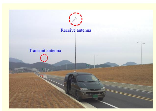
Fig. 2. Field strength measurement van.
