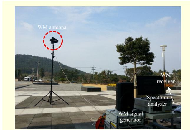
**Fig. 6.** Interference measurements from TVBD into WM receiver in front of Jeju Art Center in Korea.
