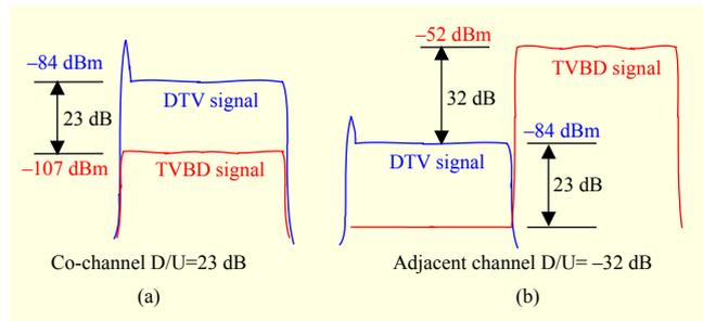
Fig. 4. (a) D/U ratio at grade B contour to protect DTV service from co-channel TVBD interference and (b) D/U ratio at grade B contour to protect DTV service from adjacent-channel TVBD interference.
