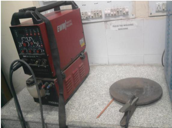
Fig. 2 Pulse TIG welding machine
