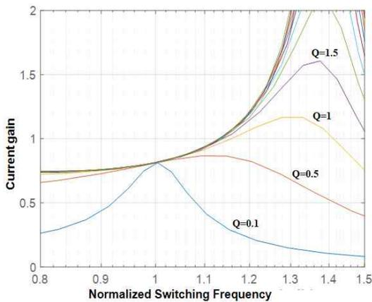
Fig. 6. Current gain (H) for  $\gamma = 1$
