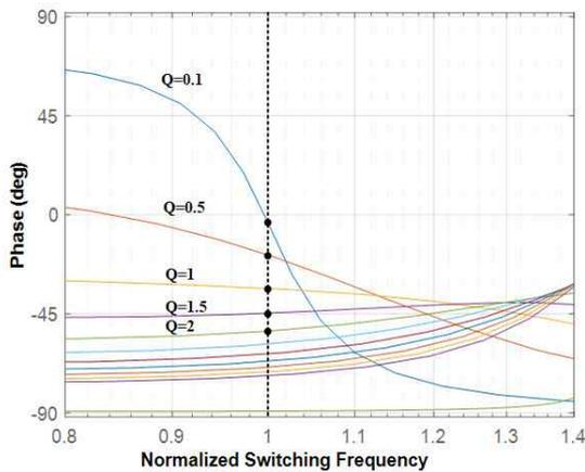
Fig. 7. Phase difference between inverter voltage and current for  $\gamma = 0.465$
