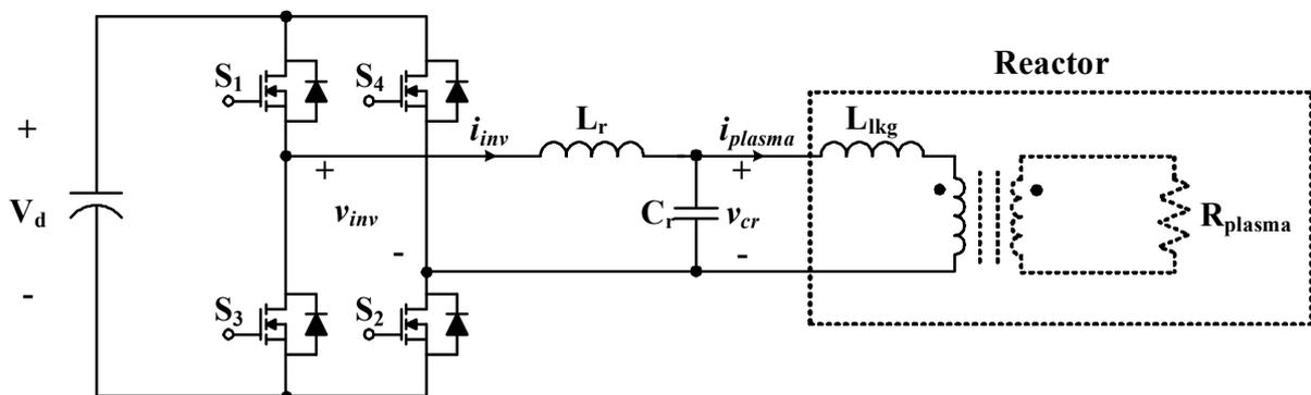
Fig. 5. Circuit diagram of resonant inverter for reactive gas generator
