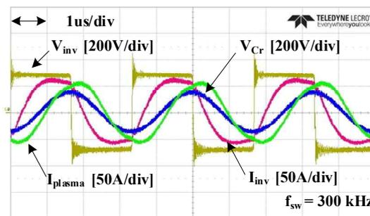
(a)  $I_{plasma}^* = 30A$ ,  $O_2 = 5$  L/min
