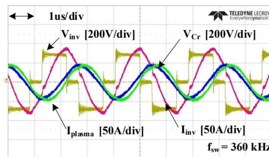
(b)  $I_{plasma}^* = 24A$ ,  $O_2 = 5$  L/min
