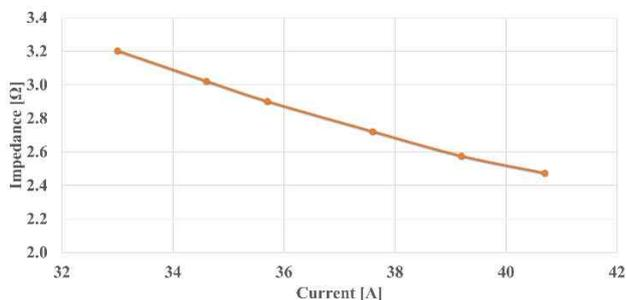
Fig. 3. Impedance of plasma load when the primary current of the reactor varies
