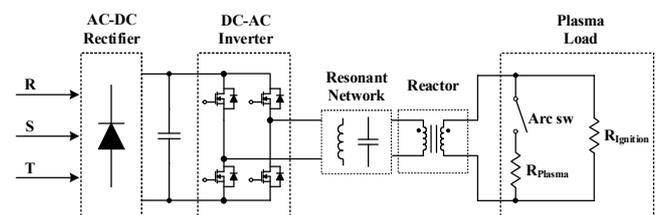
Fig. 1. Basic structure of the reactive gas generator
