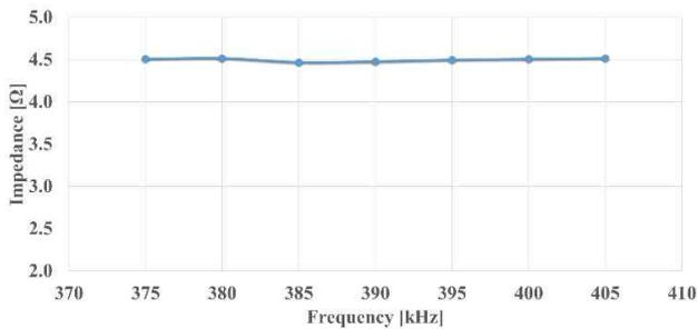
Fig. 2. Impedance of plasma load when the operating frequency varies
