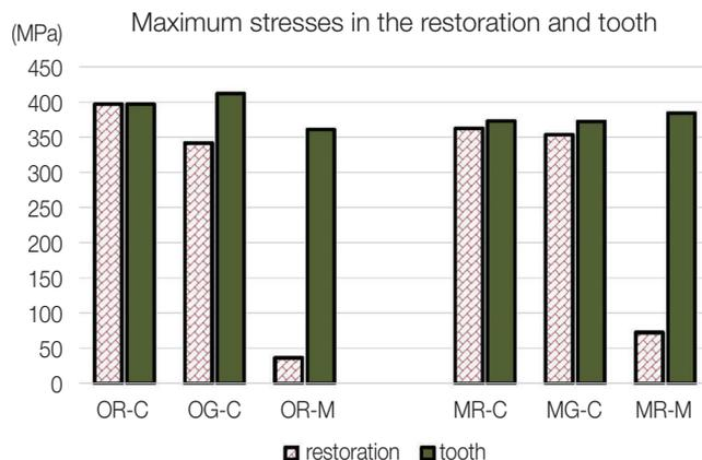
**Fig. 4.** Minimal invasive cavity designs (OR-M, MR-M) produced very small maximum von Mises stress magnitude compared to conventional inlay designs in the restoration. There were no significant differences in maximum stress magnitudes within the abutment tooth among models.
